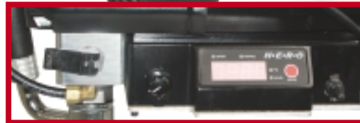
"SSPC" electronic pressure control and display
